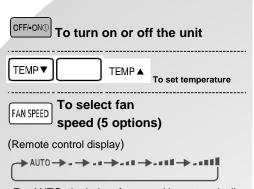
• For AUTO, the indoor fan speed is automatically adjusted according to the operation mode.
